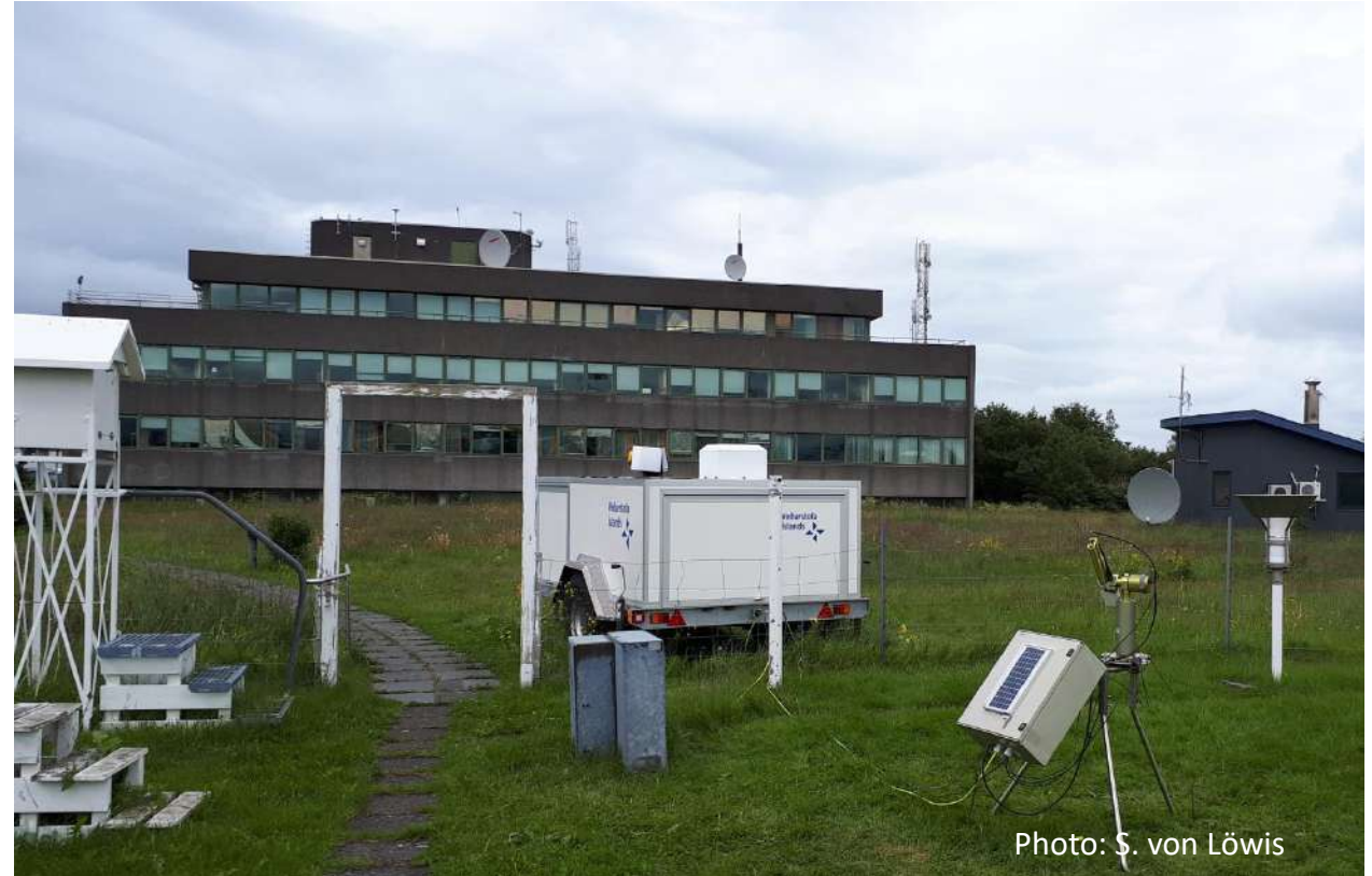
The mobile lidar/ceilometer trailer and the sun-photometer at IMO, Reykjavik.
